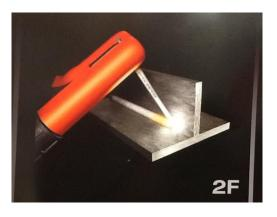
1) Jr. Division will weld both sides with a 1/8 E6010(two welds with E6010)
